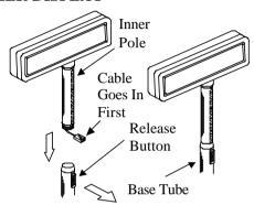
down into the base tube. Please ensure that the latching track on the inner-pole matches up with the release button. Open the back door and find the connector marked "customer display" or "VFD". Please remove the VFD terminator from this connector and store in a safe place. Insert the cable plug of the customer display into customer display connector until a click sound is heard.
